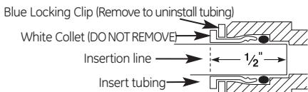
9. Pull out slightly on tubing to ensure a good seal.
